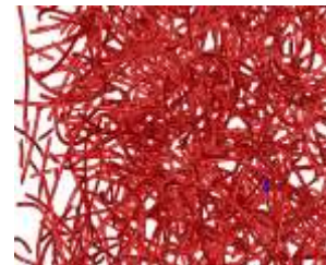
Polymer matrix reinforced with 2% (volume fraction) of carbon nanotubes
