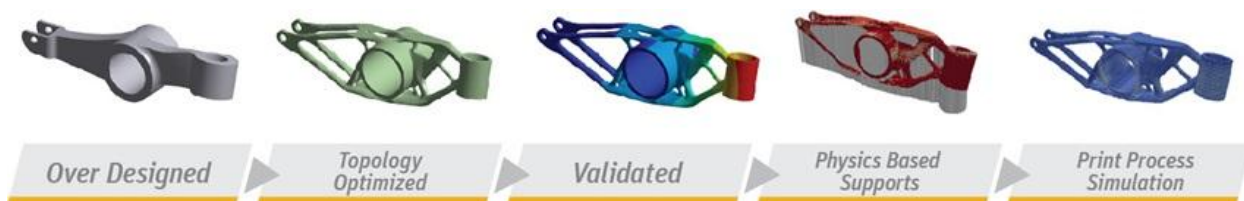
Fig: ANSYS Additive simulation process
